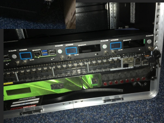
Right: Rack case showing trial installation of PDU, switch and 1U compute node unit
